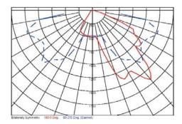
Spacing of each box is equal to mounting height in feet.
