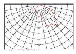
Spacing of each box is equal to mounting height in feet. Ex: 40ft mounting height = each box is 40ft, 30ft mounting height = each box is 30ft
